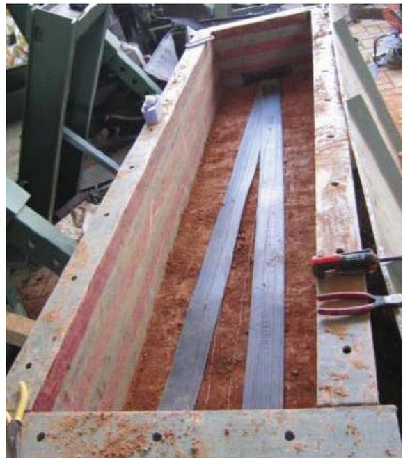
Fig. 10 Polyester strap with unanchored V-configuration in pullout box.
