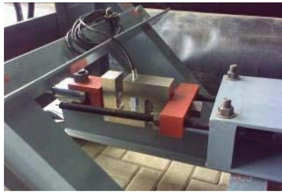
Fig. 9 Load cell installed to clamping system and hydraulic actuator.
