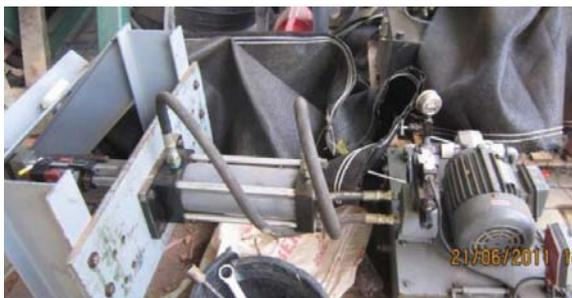
Fig. 8 Displacement-controlled pullout system.
