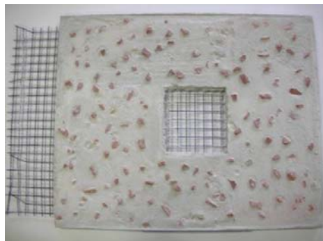
Fig. 4 Porous thin cement composite containing brick chips at the surface and fine wire mesh as the reinforcement
