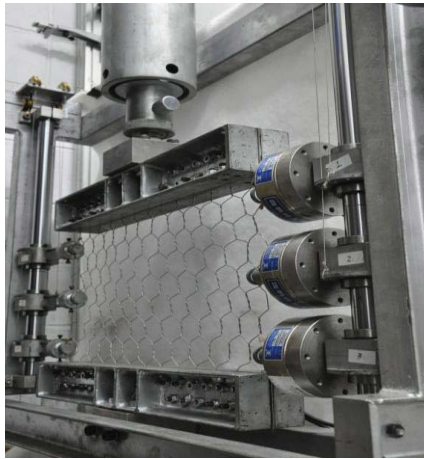
Fig. 4 Schematic view of the setup for lateral constrained tensile test.
