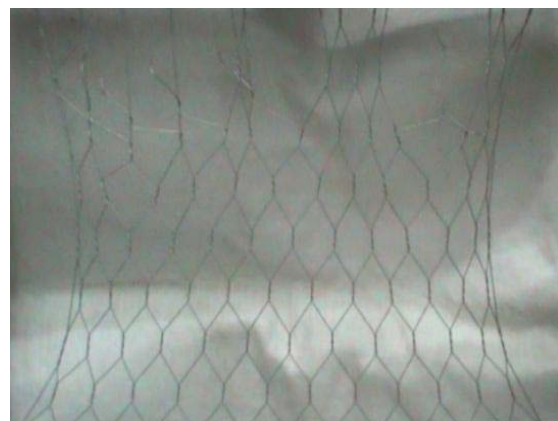
Fig. 11 Tensile failure mode of Type A mesh panel without lateral constraint (Type Au n ).
