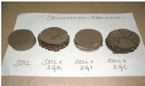
Fig. 13 View of shrunken sample of soil and soil + two layer of geosynthetics in horizontal orientation
