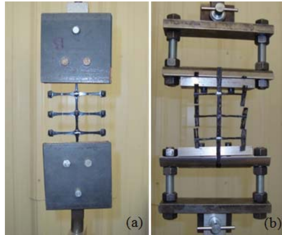
Fig. 2 Rib tensile strength test clamps modified for (a) EGG, (b) NEGG geogrids (Hatami et al. 2011.a)
