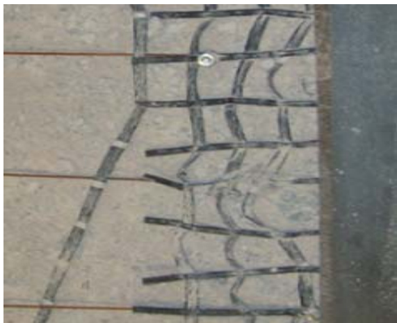
Fig. 4 NEGG-3 geogrid condition after pullout test
