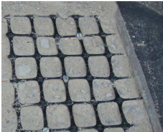
Fig. 3 EGG-1 geogrid condition after pullout test
