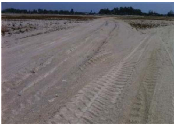
Fig. 1 The top soil comprises of very loose sand which is prone to extensive rutting
