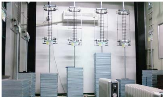
Fig. 5 Tensile creep testing machine and test set up
