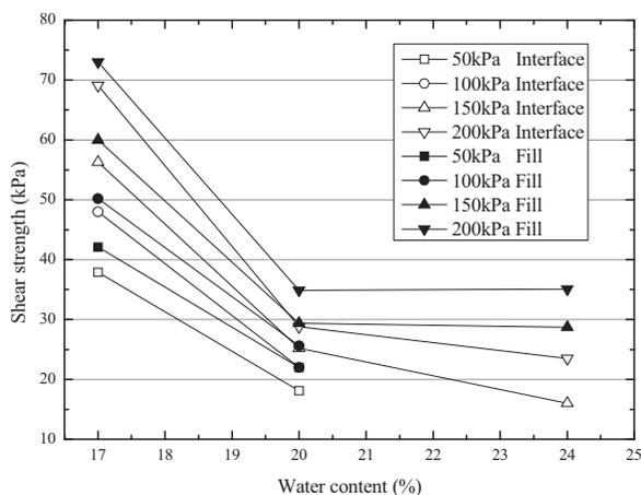
Fig. 5 The shear strength of the geogrid-soil interface and the backfill while water content increase
