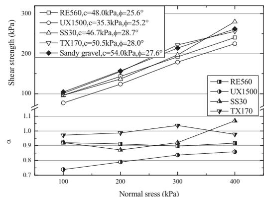
Fig. 3 The interface characteristics under different geogrids
