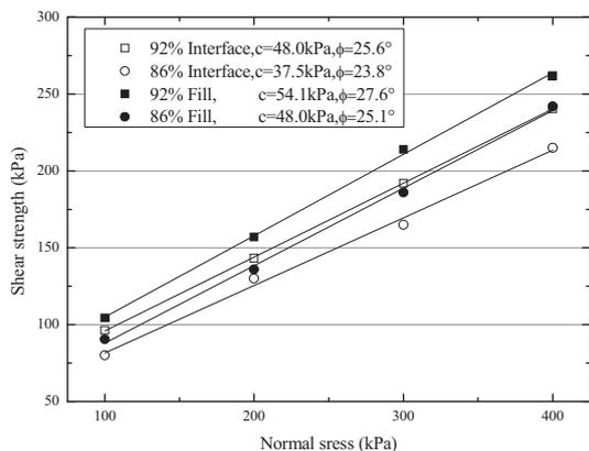
Fig. 4 The interface characteristics under different compaction degree.
