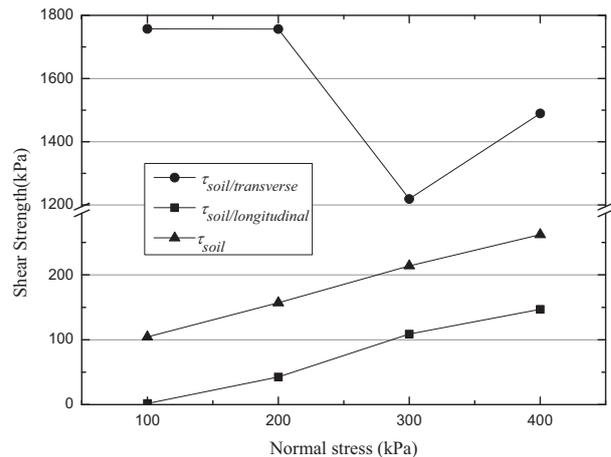
Fig. 8 Shear strength provided by the longitudinal and transverse ribs of uniaxial geogrid under different normal stress
