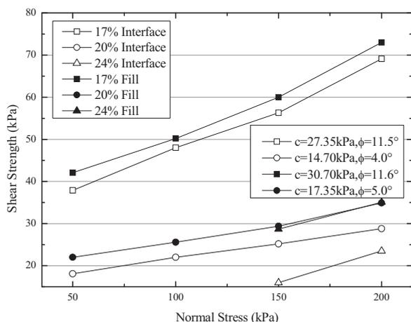
Fig. 6 The geogrid-soil interface and the backfill shear strength characteristics with different water content.
