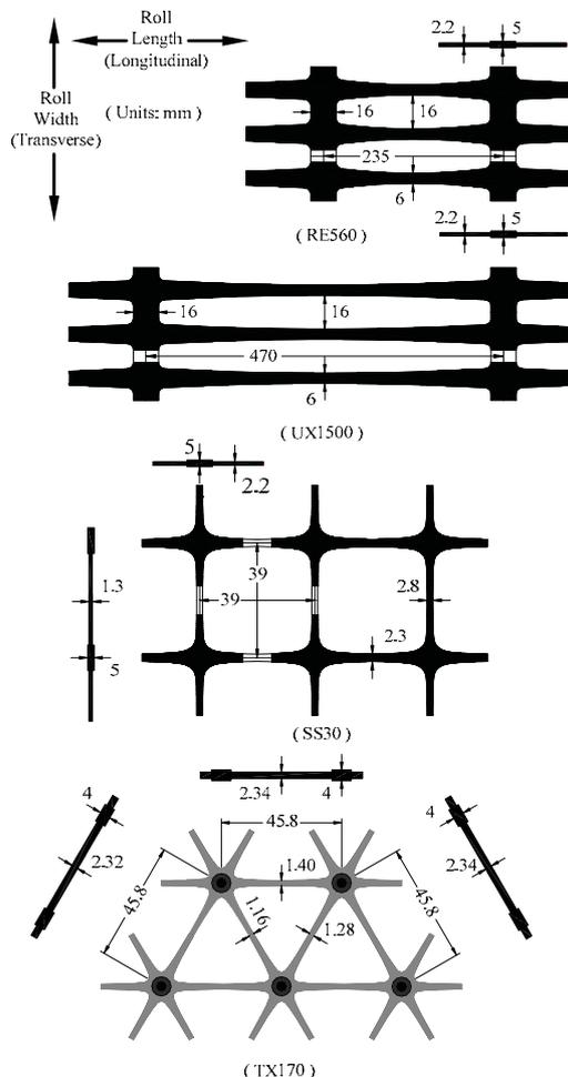
Fig. 1 Sketch of the geogrids used in the tests.
