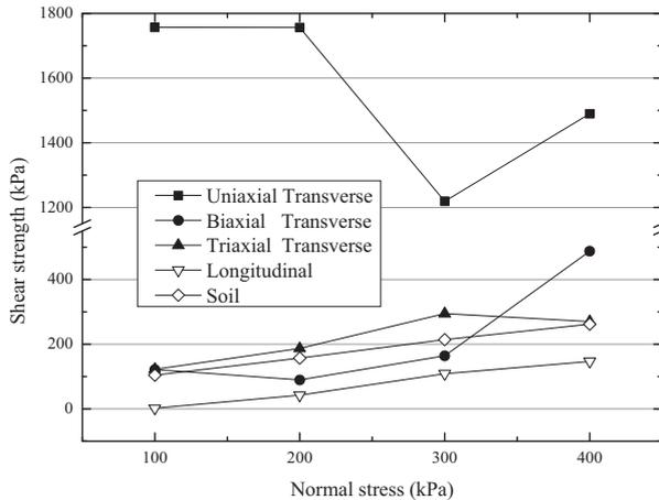
Fig. 9 Shear strength provided by the longitudinal and transverse ribs of different geogrid under different normal stress
