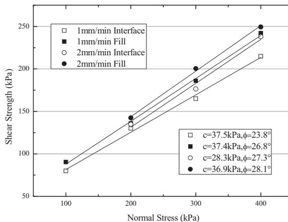
Fig. 7 The geogrid-soil interface and the backfill shear strength characteristics with different shearing rate.
