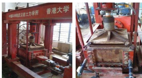
Fig. 2 Large-scale direct shear apparatus
