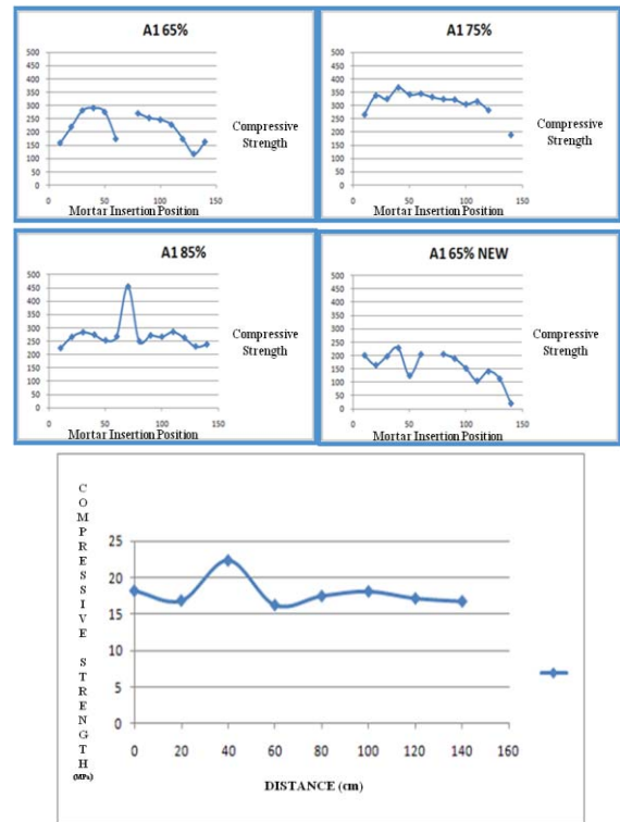
Fig. 10 Compressive strength of A1 fabric foam with water content
