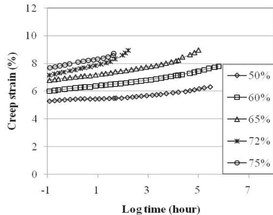
Fig. 8 Tensile creep master curve of WG-8 after installation damage by filling soil.
