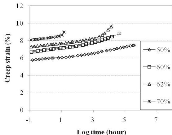
Fig. 9 Tensile creep master curve of WG-8 after installation damage by gravel.
