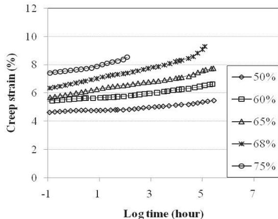
Fig. 7 Tensile creep master curve of WG-8 after chemical exposure (pH 9, 50 °C, 4 months).
