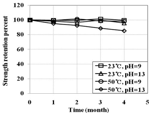
Fig. 3 Strength retention of un-notched WBG-6.
