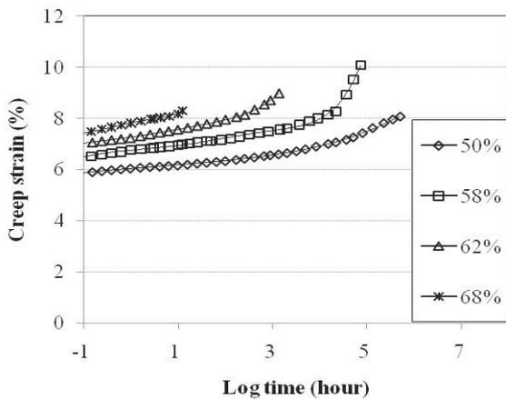
Fig. 11 Tensile creep master curve of WG-8 after installation damage and chemical exposure (pH=9, 50°C, gravel).
