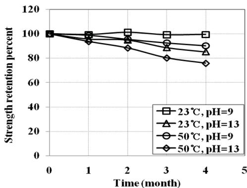
Fig. 4 Strength retention of notched WBG-6.
