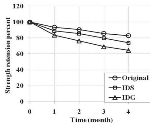
Fig. 6 Rib tensile strength retention percent of WG-8 with exposure conditions (pH 13, 50°C).
