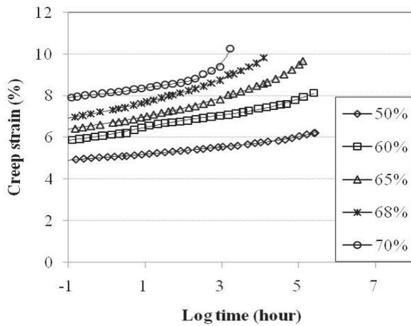
Fig. 10 Tensile creep master curve of WG-8 after installation damage and chemical exposure (pH=9, 50°C, soil).
