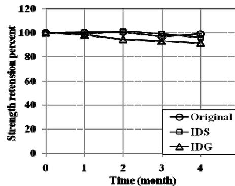
Fig. 5 Rib tensile strength retention percent of WG-8 with exposure conditions (pH 9, 50 °C).
