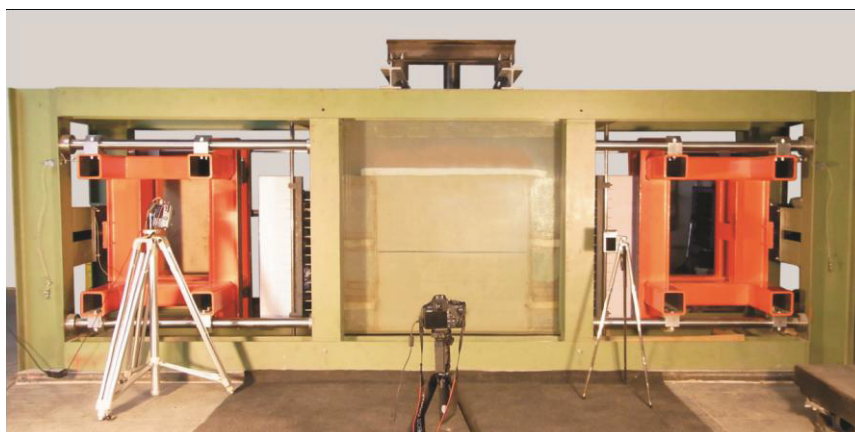
Fig. 1 Laboratory apparatus for large scale biaxial compression testing and sketch of the specimen.
