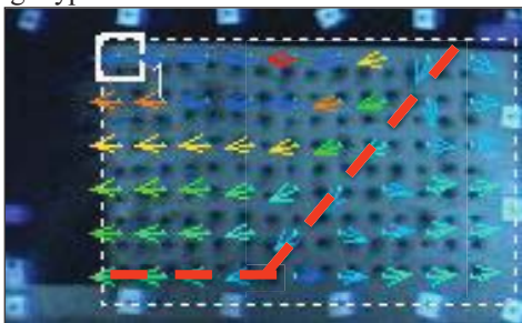
Fig. 7a Potential sliding surface before the collapse
