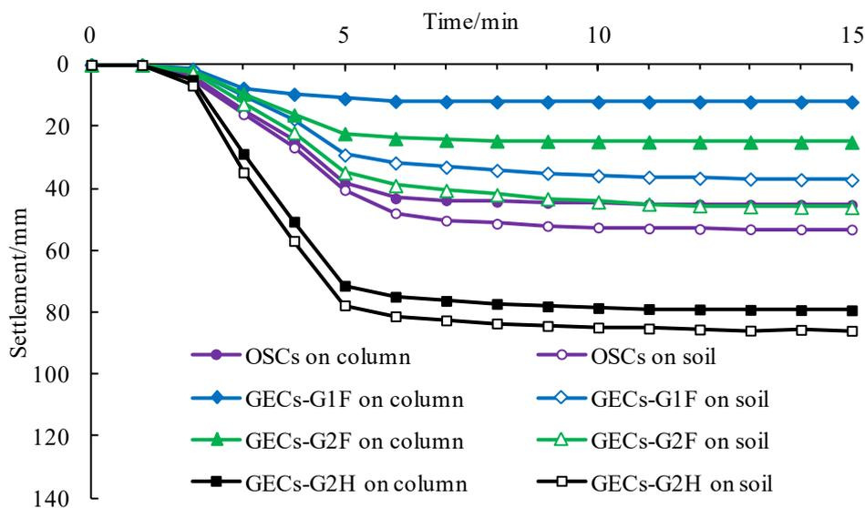
Figure 3. Settlement on the top of columns and soil
