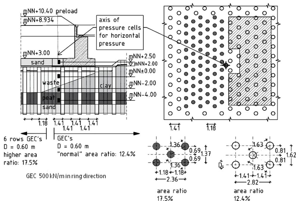
Figure 3. GEC foundation near the abutment: longitudinal cross-section (left) and plan view (right); mNN=average sea level
