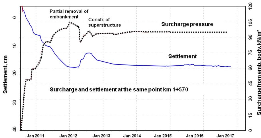
Figure 4. Typical settlements at level mNN+3.00 (see Figure 3, left)
