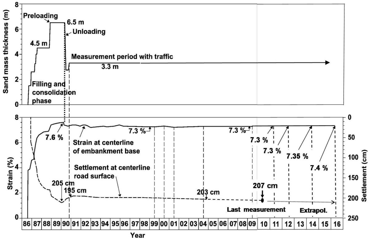
Figure 1. Grossemeer highway embankment over 30 years (1986 - 2016): embankment height, settlements and strains in the basal reinforcement.
