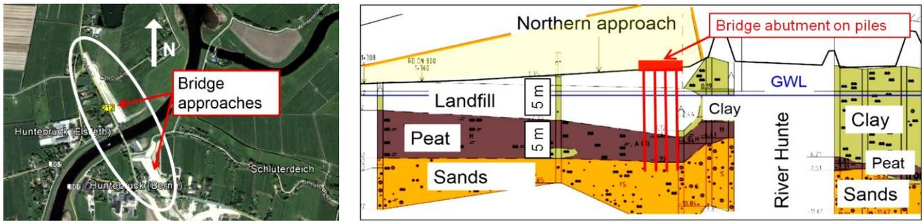
Figure 2. Berne bypass: Overview of crossing the river Hunte (left) and simplified longitudinal cross section (right); GWL=average ground water level
