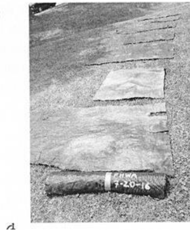
Figure 8. Exhumed and cleaned geotextiles
