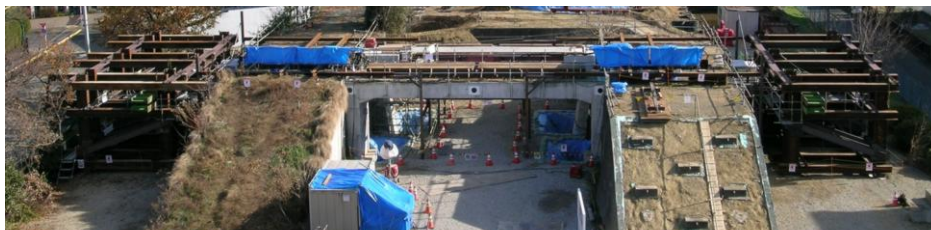
Figure 3. A general view of the model with arrangements for lateral cyclic loading tests (Koda et al., 2013).
