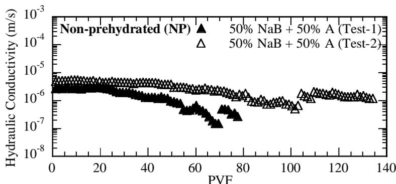
Figure 3. Hydraulic conductivity of non-prehydrated 50%NaB+50%A GCLs as a function of pore volumes of flow.
