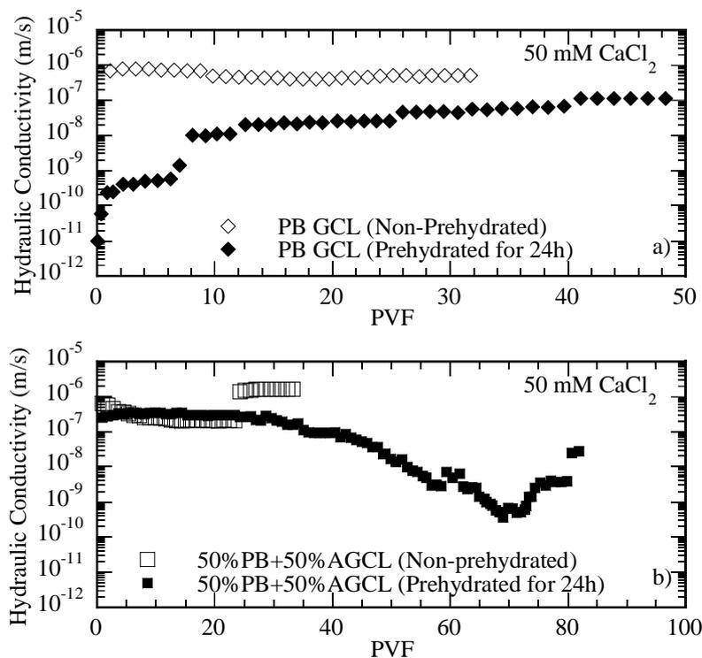
Figure 6. Comparison of the hydraulic conductivity of non-prehydrated and prehydrated GCLs when permeated with 50 mM  $\text{CaCl}_2$  solutions: a) PB GCL and b) 50%PB+50%A.
