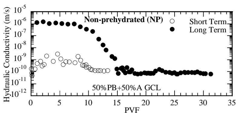
Figure 2. Comparison of the short and long-term hydraulic conductivities of non-prehydrated 50%PB+50%A GCLs as a function of pore volumes of flow.
