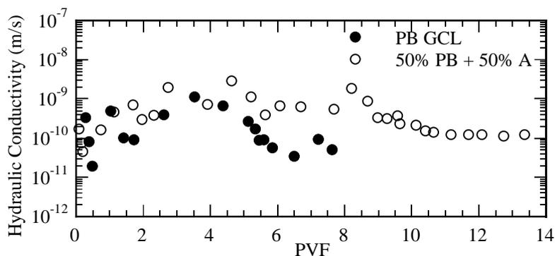
Figure 1. Hydraulic conductivity of non-prehydrated PB and 50%PB+50%A GCLs as a function of pore volumes of flow (PVF).
