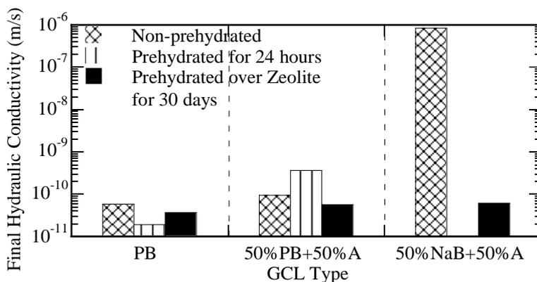
Figure 5. Comparison of the hydraulic conductivities of GCLs in terms of prehydration.
