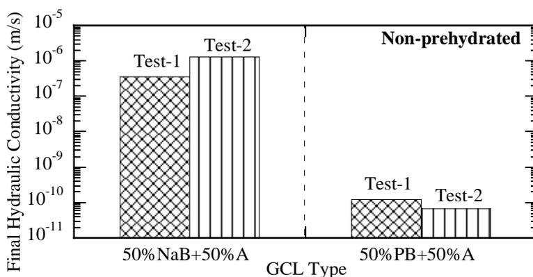
Figure 4. Comparison of the hydraulic conductivities between 50%NaB+50%A and 50%PB+50%A GCLs.
