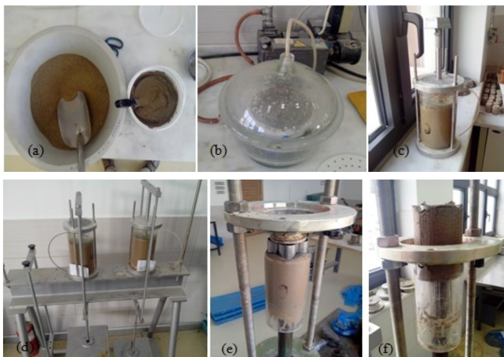
Figure 4. Preparation of soil samples (a, b) Saturation phase (c, d) Consolidation phases (e, f) Soil extraction
