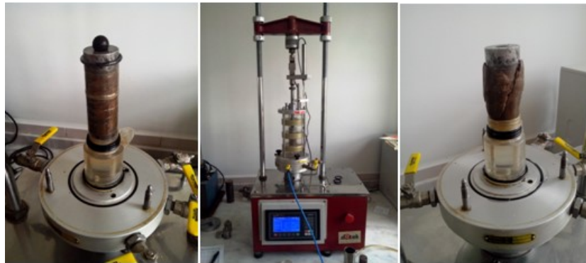
Figure 5. Unconsolidated undrained triaxial tests (UU)
