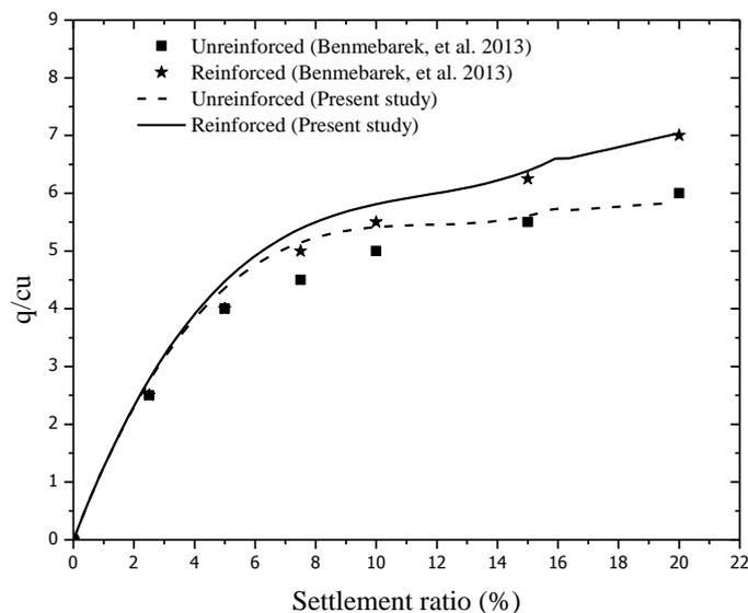
Figure 3 Plot showing comparison of settlement ratio and normalised load of present study with literature
