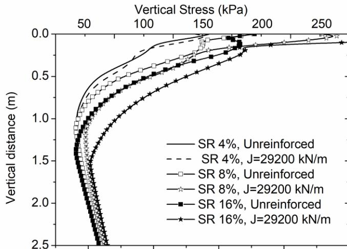
Figure 8 Variation of vertical stress with depth in unreinforced and reinforced pavement system at different levels of settlement ratio (SR)
