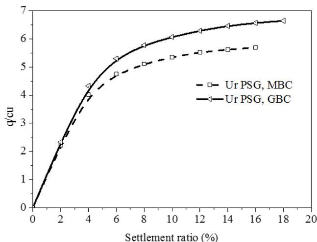
Figure 4 Variation of bearing pressure with settlement ratio for unreinforced pavement with good base course and marginal base course
