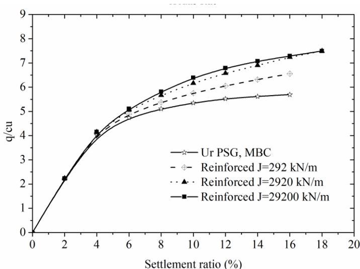
Figure 5 Variation of load with settlement ratio for unreinforced and reinforced pavement with marginal base course
