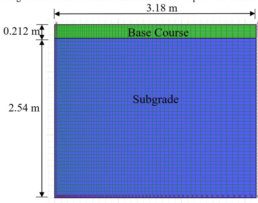
Figure 2 Graded mesh geometry with pavement layers and dimensions used in FLAC2D
