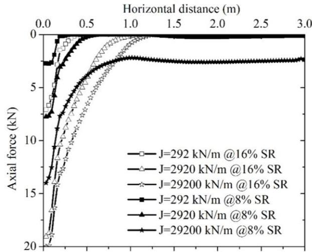
Figure 6 Variation of axial force in reinforcement with horizontal distance at settlement ratio of 8% and 16%
