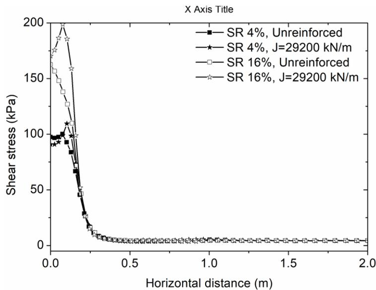
Figure 10 Shear stress profile along the subgrade surface at 4% and 16% settlement ratios with and without reinforcement
