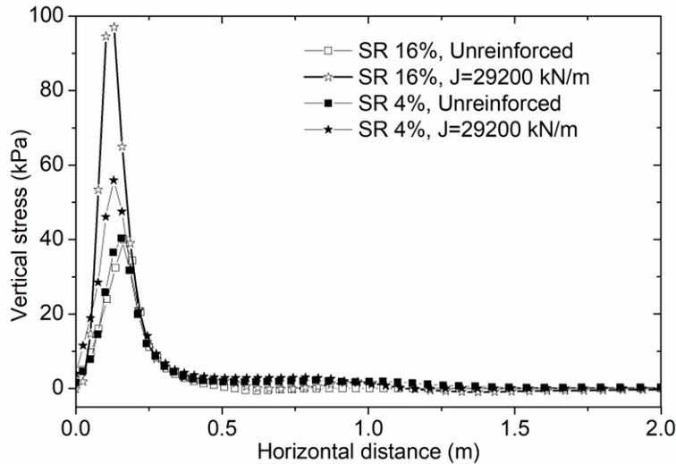
Figure 9 Vertical stress profile along the subgrade top at 4% and 16% settlement ratios of unreinforced and reinforced pavement system
