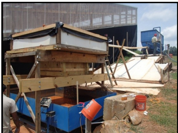
Figure 11. D7351 modified for inlet testing.
