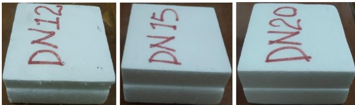
Figure 4. The observed shear of EPS geofilm test specimens for different densities.
