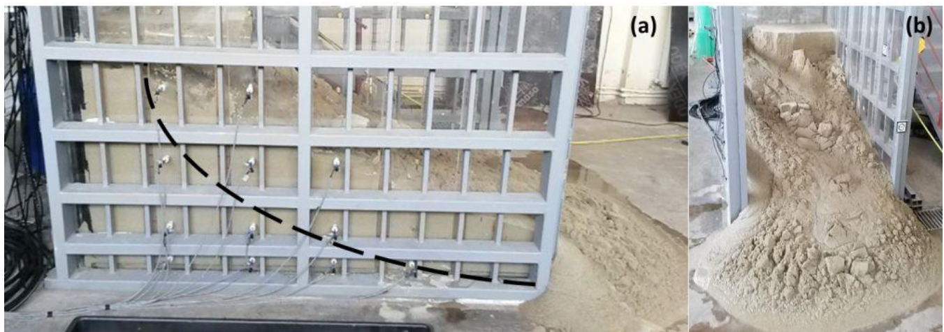
Figure 4. Physical condition of the matrix embankment at the end of the test (a) Side view of the failure surface with hypothesized rotational failure plane entering at the crest and exiting at the toe (b) Front view of the failure surface (Akay et al., 2016)
