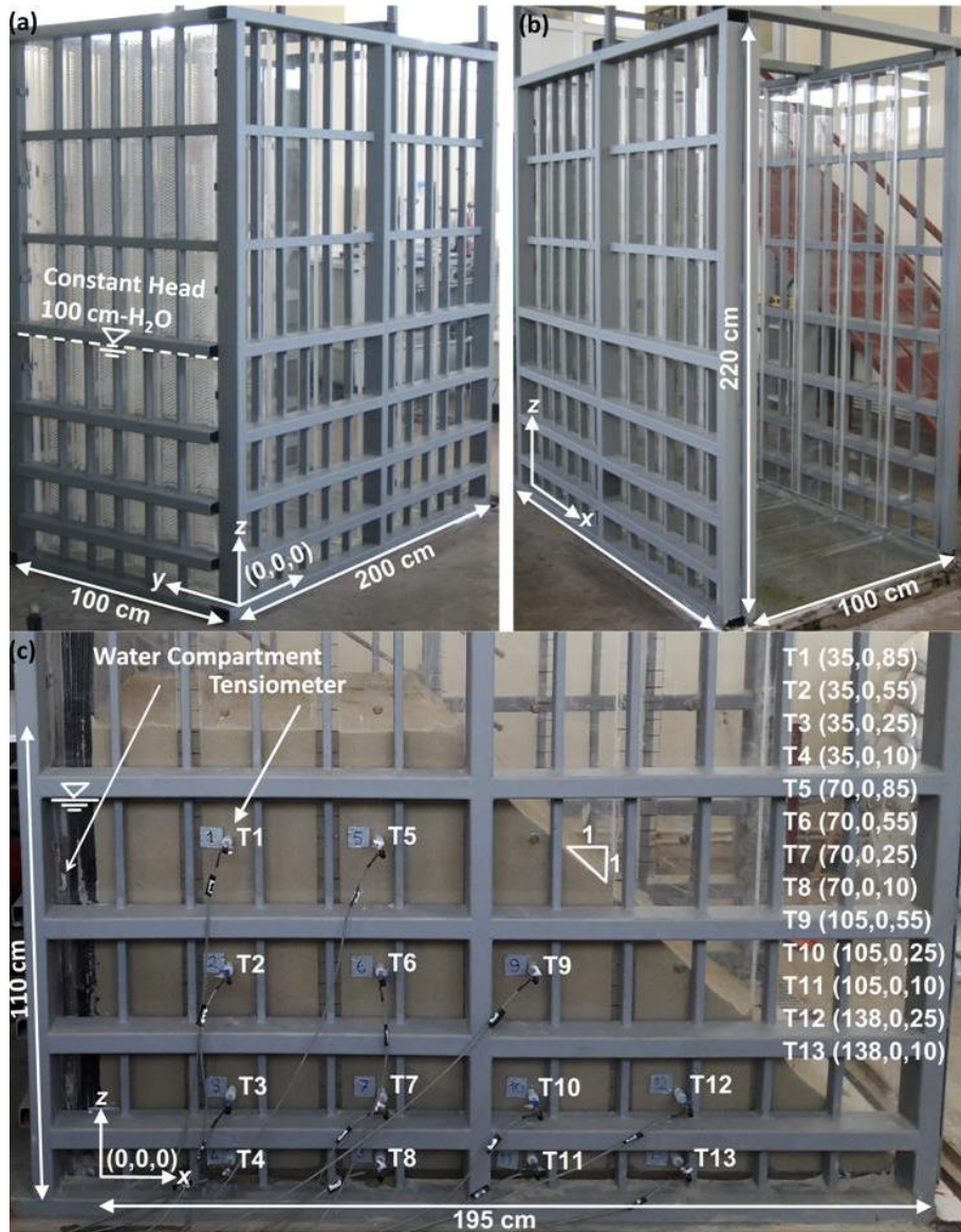
Figure 1. Laboratory test bed (a) Plexiglas test bed with steel frame (a) Plexiglas test bed with steel frame, alternative view (c) Embankment model and location of tensiometers (Akay et al., 2017).
