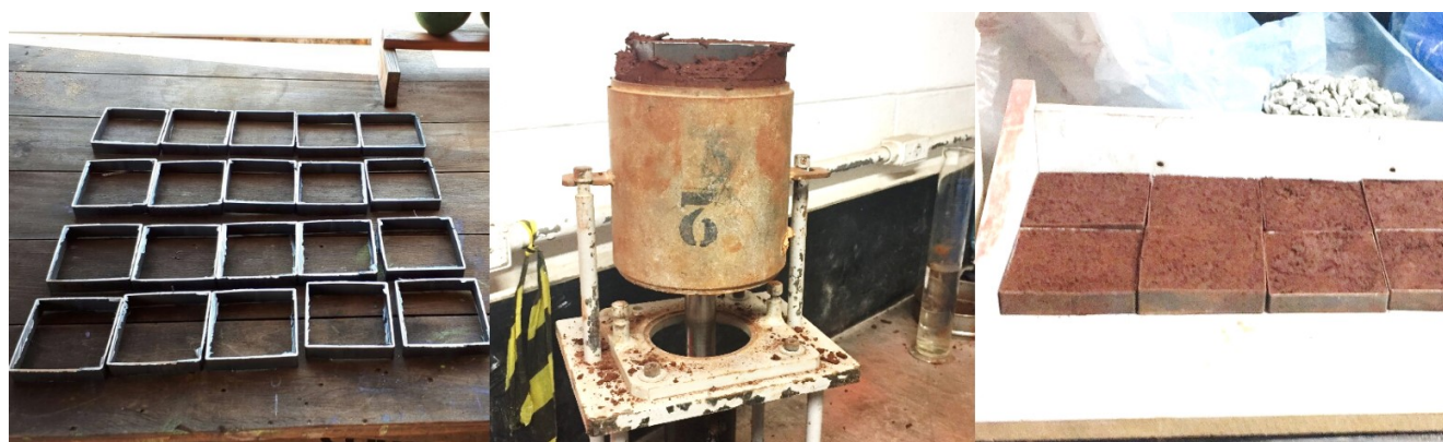
Figure 3(a). The molds (100x100mm). (b) The molding process. (c)The molded samples
