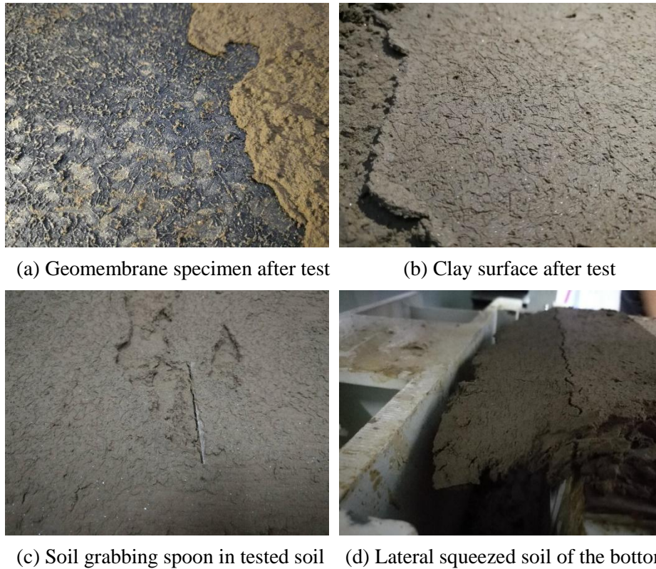
Figure 7. Visual inspection of the specimens after test.
