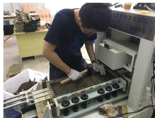
(c) Compacting the tested soil
