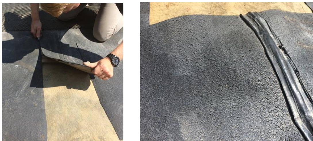
Figure 5. Field sampling of sheet removal and various seams.
