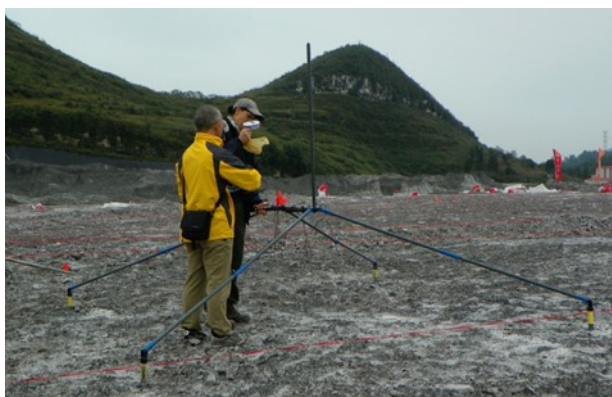
Figure 15 Dipole (quadrapole) test in progress
