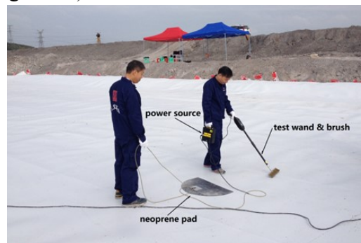
Figure 14 Spark testing in progress
