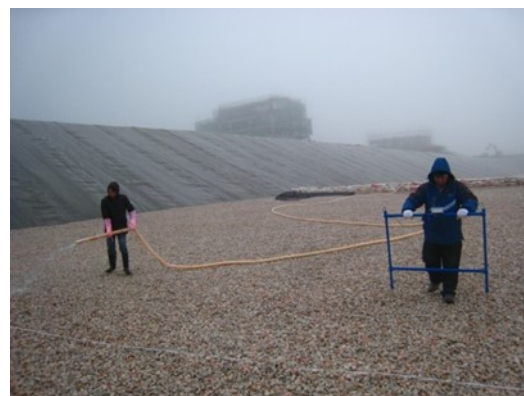
Figure 10 Dipole test at bottom
