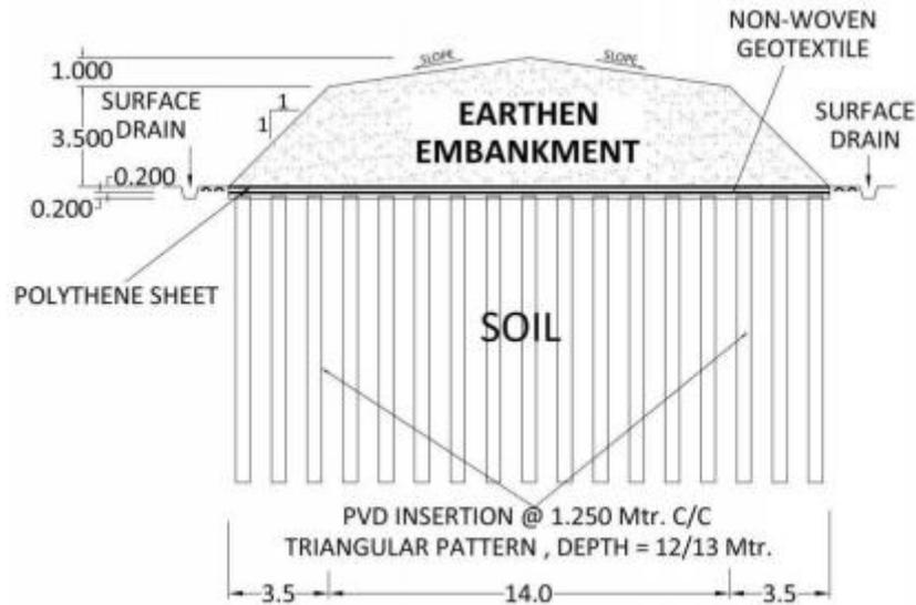
Figure 2: Cross Sectional details of PVD
