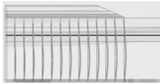
Figure 11: Deformed shape of vertical drain
