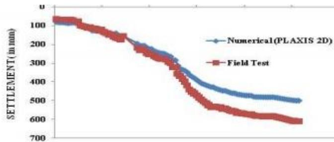
Figure 13: Validation of field investigation with numerical analysis of Settlement vs. Time at centre position
