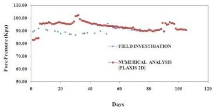
Figure 14: Validation of field investigation with numerical analysis of Pore Pressure vs. Time at centre position
