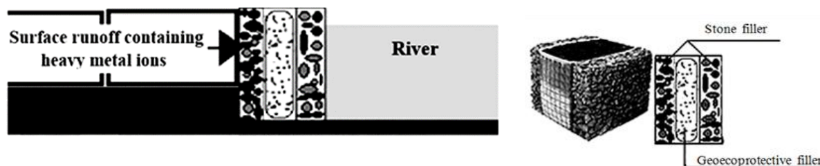
Figure 1. Gabion construction with stone and geocoprotective loading.
