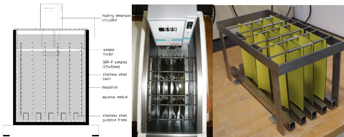
Figure 3. Test setup and photos of test equipment (picture: BAST).
