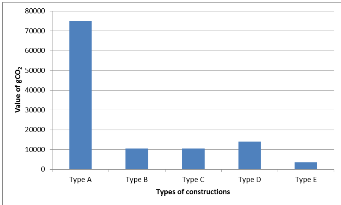
Figure 2. The value g of CO 2 in the extraction and production of raw materials and products of different types of terrace / retaining walls.
