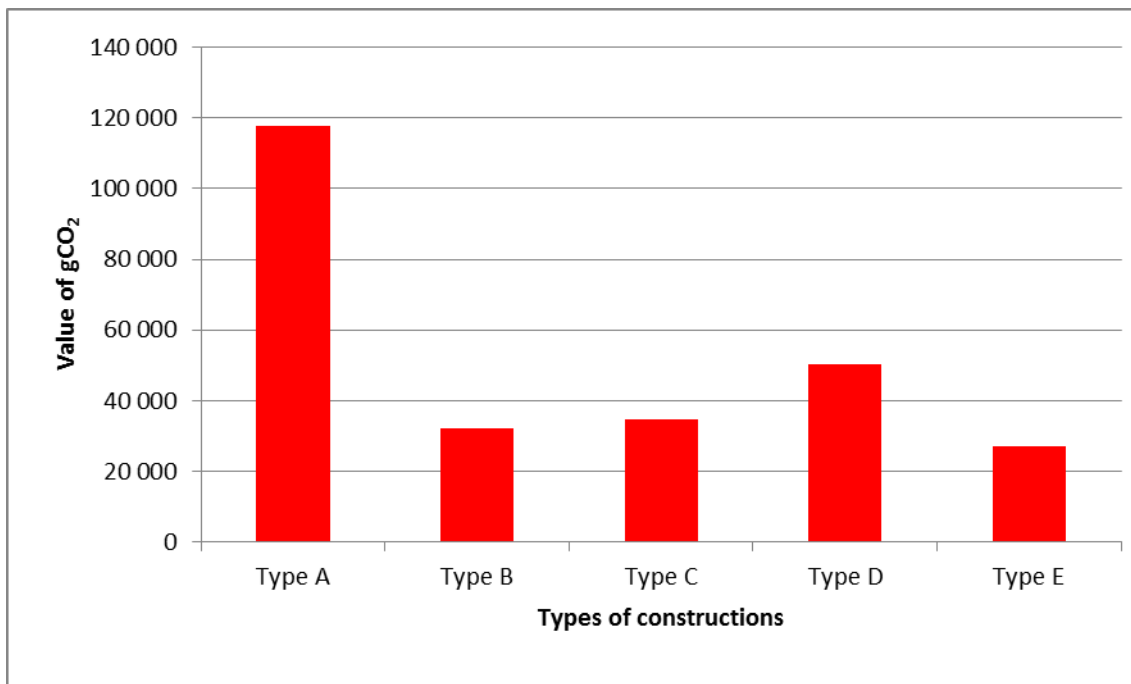
Figure 5. The total value of gCO 2 for all the processes of different types of terrace / retaining walls including earthworks.
