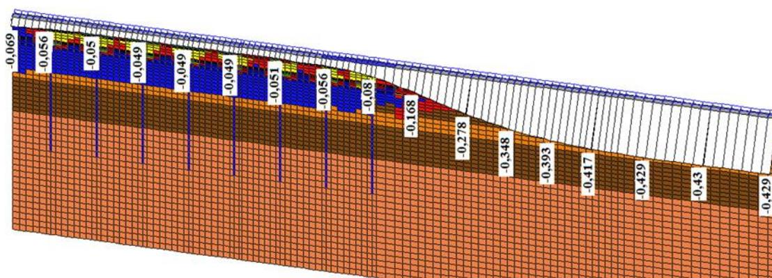
Figure 7. Curve of vertical deformation on construction surface of with variable stiffness design, m.
