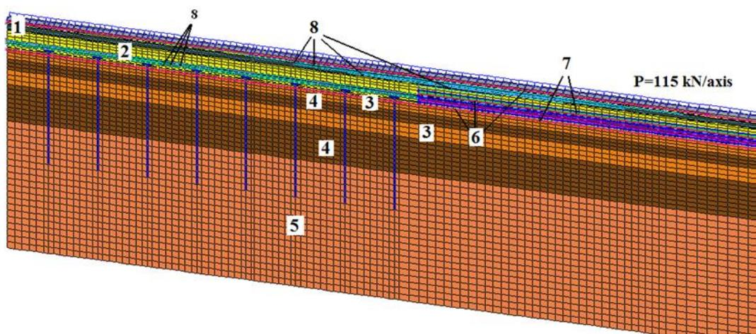
Figure 5. Numerical model: 1 – pavement; 2 - crushed stone; 3 – silty sandy loam; 4 – silt loam; 5 – pebble; 6 – biaxial geogrid E'GRID 3030L; 7 – geotechnical holder from uniaxial geogrid E'GRID 170R(L) ; 8 – biaxial geogrid E'GRID 4040L.
