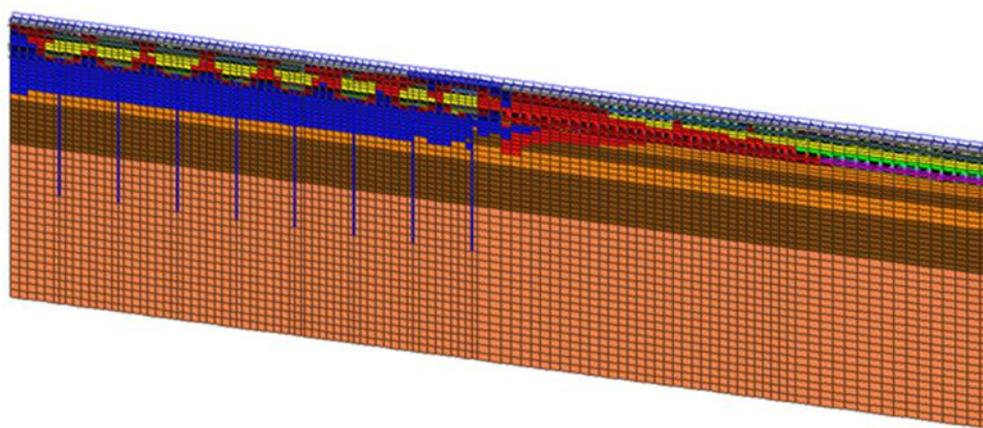
Figure 6. Zones of elastic and plastic deformations: blue color – elastic deformations; red color - plastic deformations.
