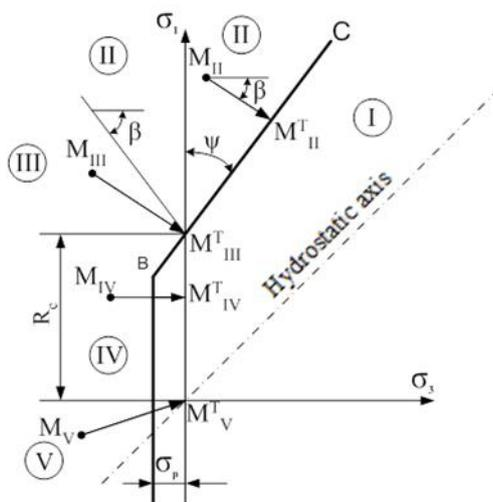
Figure 4. Scheme of determining theoretical stresses in elastic-plastic model of soil.
