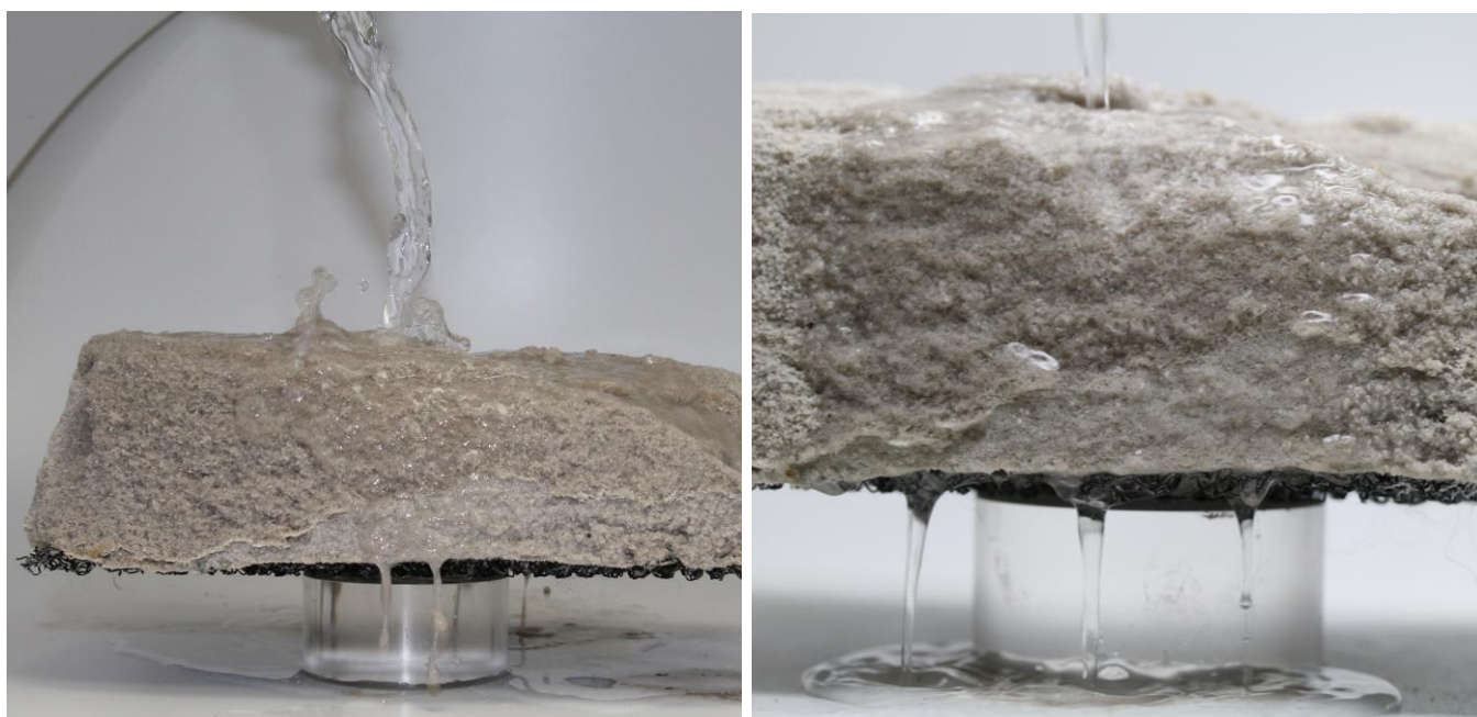
Figure 4. A 15cm-thick sand block, which was cemented via the bio-stabilization agent through the geosynthetic layer (8 mm-thick) at its bottom, resisting erosion under pressurized flow while retaining its permeability.
