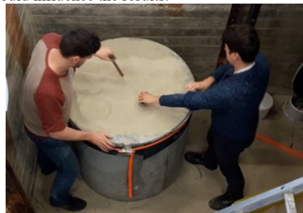
Figure 3. Loosening of the sand before an impact test by turning around wooden sticks.
