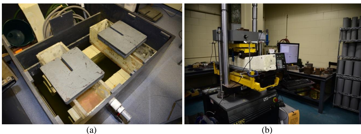
Figure 3. (a) Beam sample saturation and (b) four-point beam testing frame
