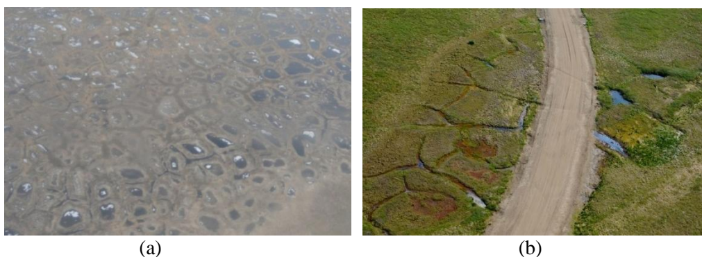
Figure 1. Examples of permafrost terrain: (a) Polygonal pattern ground with ice wedges and (b) a highway section crossing ice wedges (courtesy of Don Haley)
