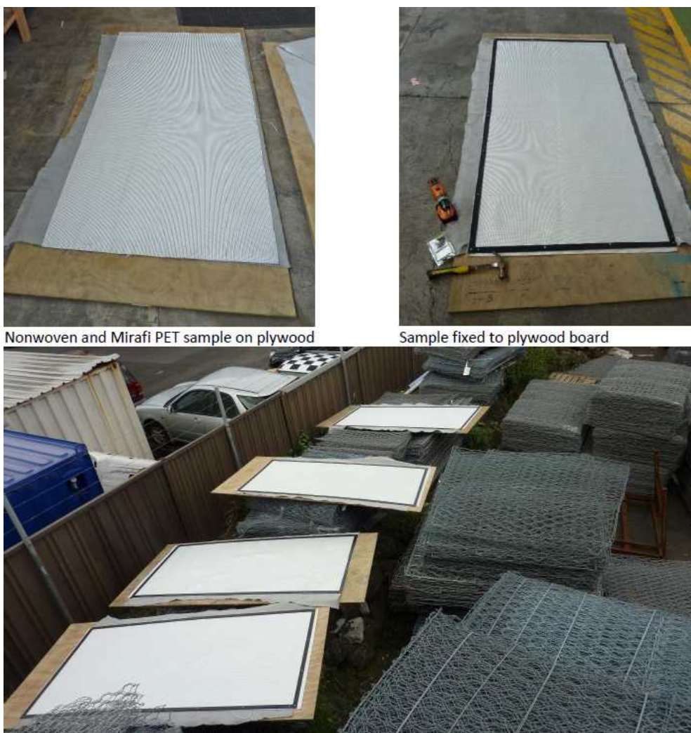
Figure 2. Geotextile sample preparation process for exposure at the Auckland yard.
