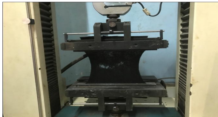
Figure 2. Testing of 150 GSM geotextile.
