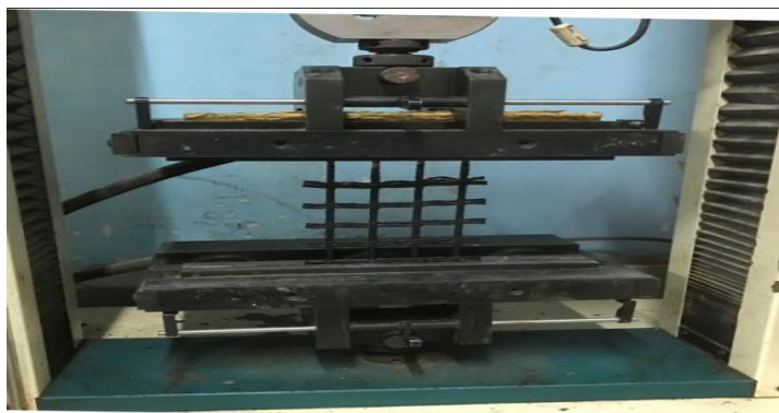
Figure 4. Tensile strength test setup for Polymer geogrid (BX 80).
