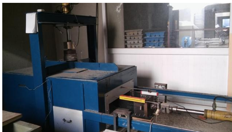
Figure 2. Photograph of pullout test box
