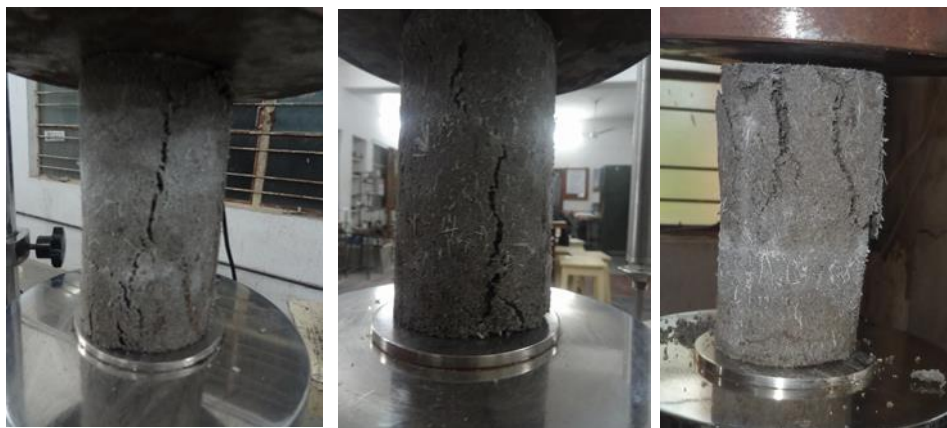
Figure 4. Failure pattern under compressive strength test
