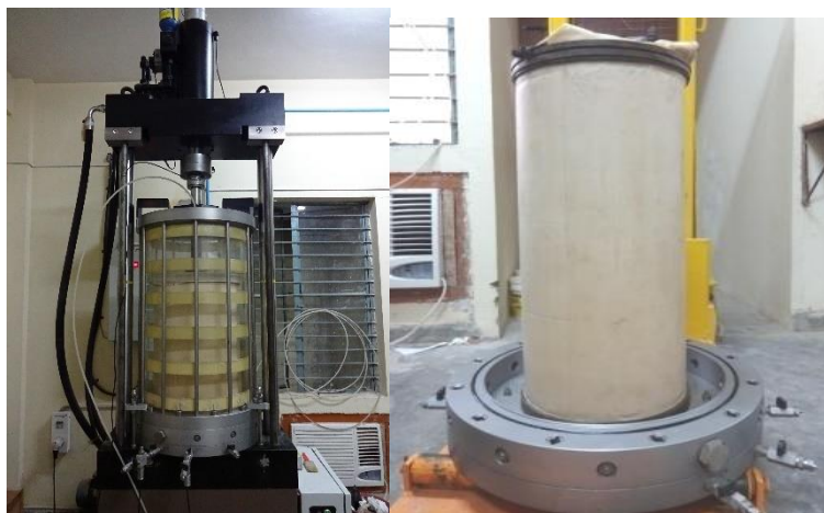
Figure3. Triaxial set-up and prepared 300 mm diameter unreinforced specimen
