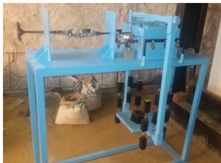
Figure 3. Shear Box with attachment for prestressing the geogrid
