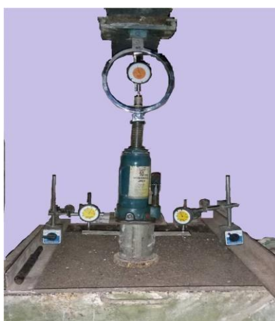
Figure 3. Plate load test set up
