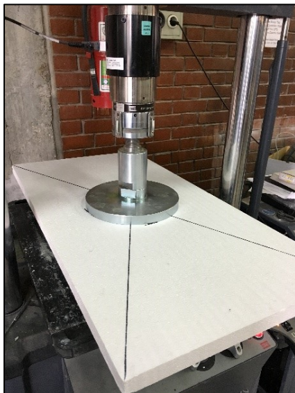
(a) (b) Figure 2. (a) Compression tests on EPS geofoam plates, (b) Stress-strain graphs of EPS plates
