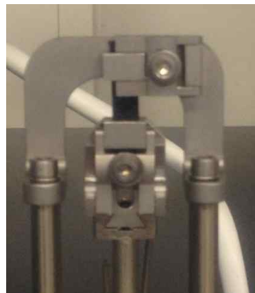
Figure 4. Specimen setup for CTE measurement, using tension clamps.
