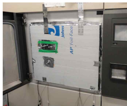
Figure 2. Insulation board closing the Xenon-arc chamber.
