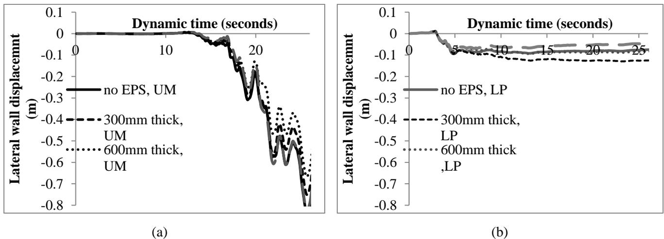
Figure 4. Displacement profile at top of the wall for (a) Umbria Marche, 1997 (b) Loma Prieta, 1989
