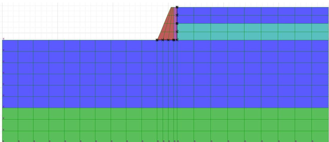
Figure 2. Meshed model in FLAC 2D
