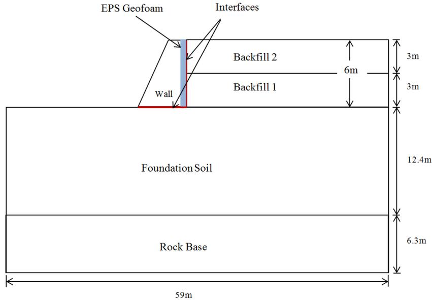
Figure 1. Schematic diagram of the model with EPS inclusion
