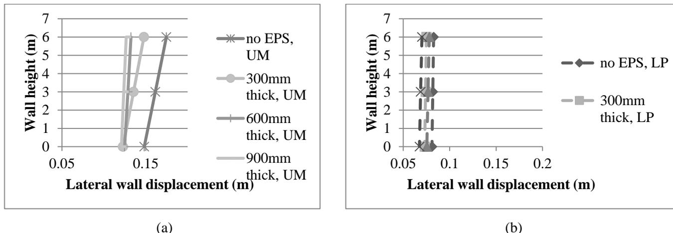
Figure 5. Displacements along the height of the wall for (a) Umbria Marche, 1997 (b) Loma Prieta, 1989
