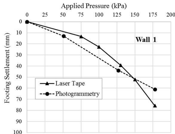
Figure 6. Pressure-Settlement Curve for Wall 1
