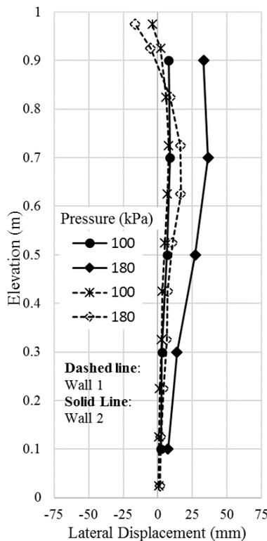
Figure 10. Comparison of Measured Lateral Displacements of Wall 1 and Wall 2
