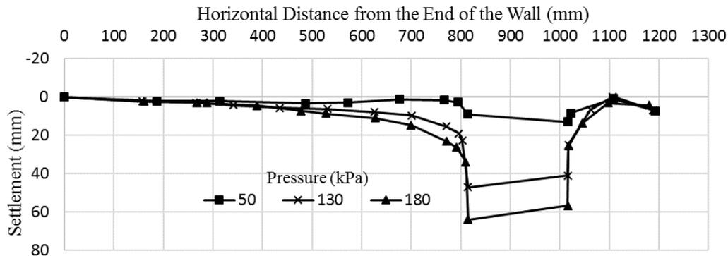
Figure 5. Settlement profiles under footing loads for Wall 1
