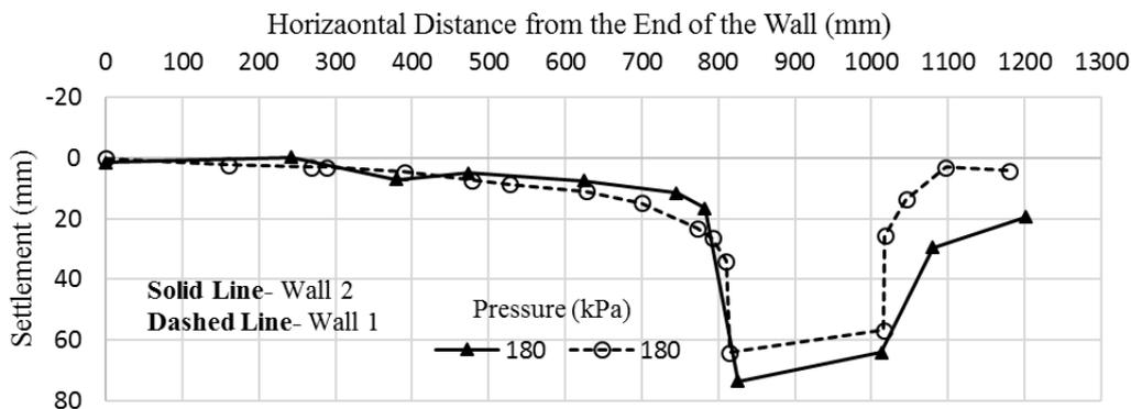
Figure 11. Comparison of Settlement profiles under Footing Loads for Wall 1 and Wall 2
