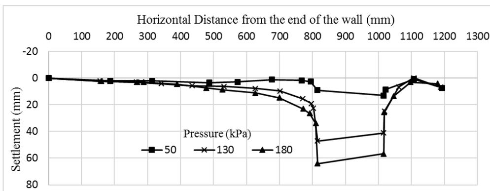
Figure 8. Settlement profiles under footing loads for Wall 2
