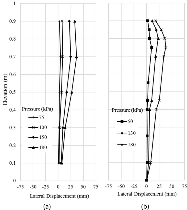
Figure 7. Measured Lateral Displacement of Wall 2 by: (a) Laser Tape and (b) Photogrammetry
