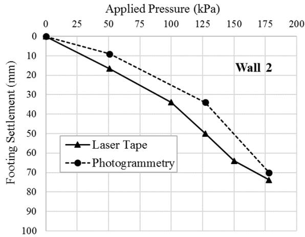
Figure 9. Pressure-Settlement Curve of Wall 2
