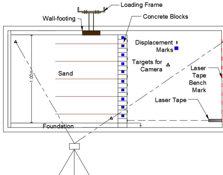
Figure 3. Camera and Laser Tape Setup
