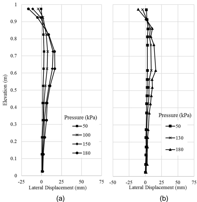
Figure 4. Measured Lateral Displacements of Wall 1 by: (a) Laser Tape and (b) Photogrammetry
