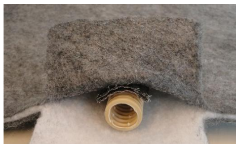
Figure 3. eGCP prototype with Geotextile A and tin-plated copper braid electrode.
