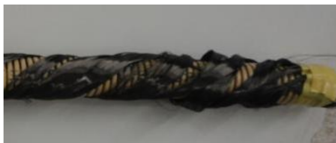
Figure 4. Carbon fiber tows wrapped around the drainage pipe.
