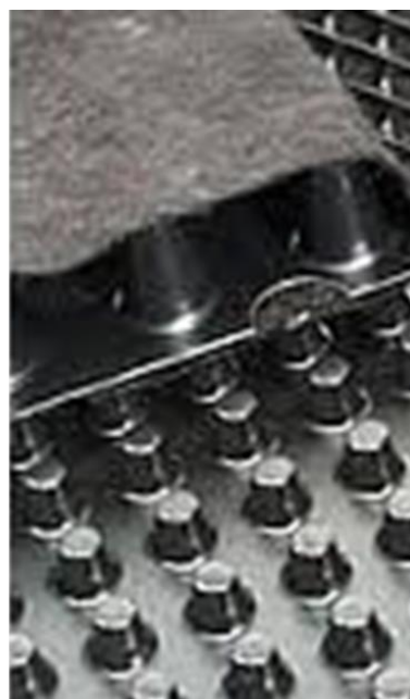
(b) Protruding columns and cuspatations of geospacers can often interlock together
