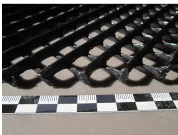
(a) Geonets - biplanar and triplanar types
