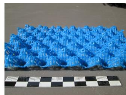
Figure 1. Various types of geonet and geospacer drainage cores.
