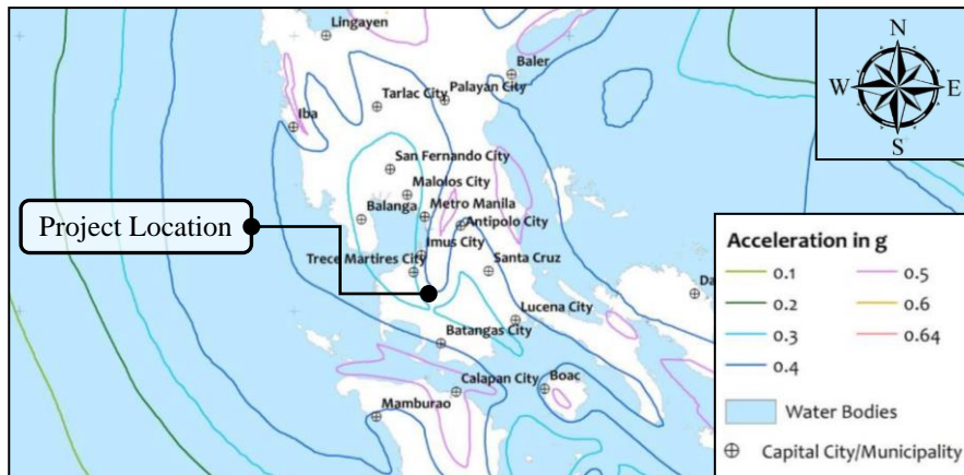
Figure 6. Extract from Peak Ground Acceleration Map of the Philippines for 500-yr Return Period on Stiff Soil (PHIVOLCS)
