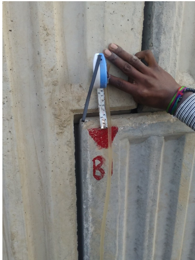
Figure 8 Settlement monitoring example
