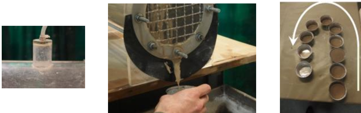
Figure 3. During the process of the test, passing sludge is regularly measured to evaluate the fines passing through the geotextile;
