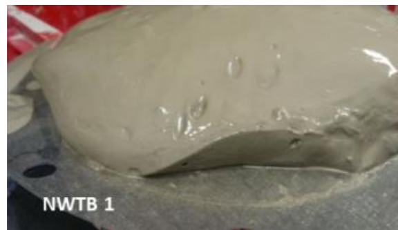
Figure 8. Cake formed with NWTB-1 in the constant head process, soil B C_s = 500 g/L.
